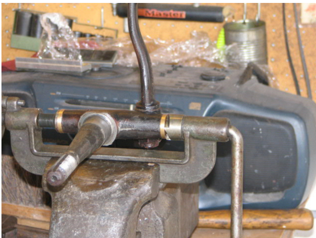
Rod Prinsen's awesome spindle bushing facer No more front end shimmy here!
